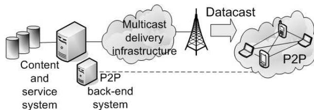
Figure 1: Combined multicast and P2P content distribution system
